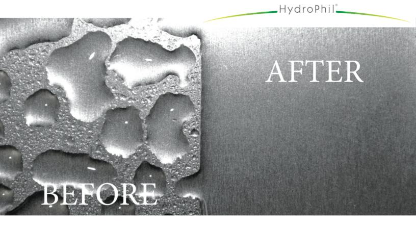
New ultra-thin coating delivers significant improvement in evaporator condensate removal without carryover Increase air velocity up to 26% over an uncoated fin
